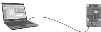
Fig. 17 CIM 500 connected to PC via Ethernet cable
