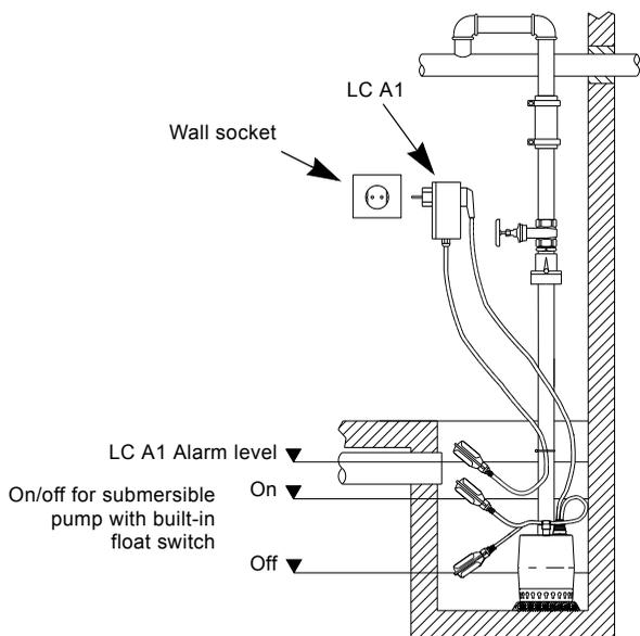
**Рис. 3** Installation with submersible pump in sump
